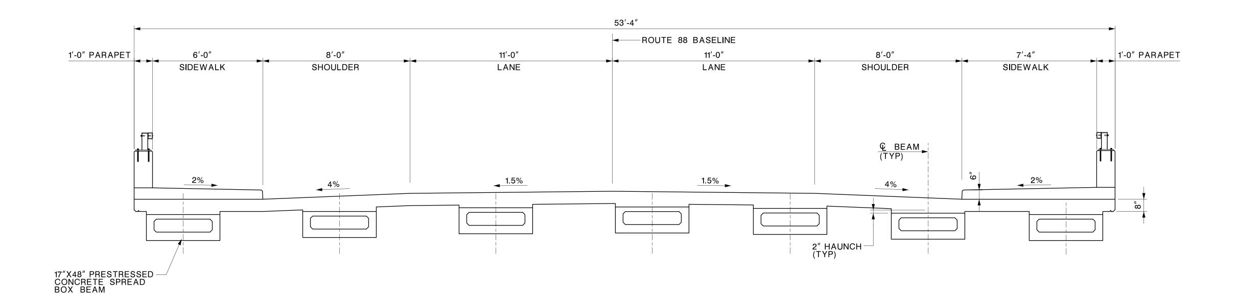
TYPICAL CROSS SECTION SCALE:  $\frac{3}{8}$ "=1'-0"
